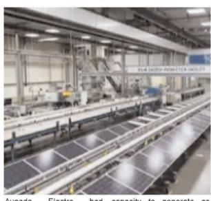
Avaada Electro groundbreaking ceremony for its Butibori plant last October Modules are the equipment that generate solar power. They are made of numerous solar cells. So far, modules made in India have smaller 182x183mm M10 cells which can generate 595Wp solar power. Avaada has begun manufacturing made of 220x220mm G12
